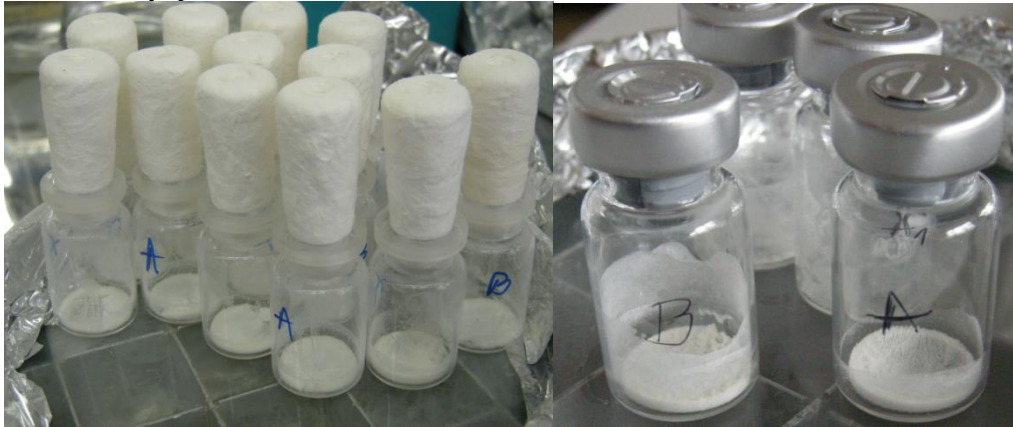
Figure 5. Lyophilized vials of Lb. plantarum (A) and Lb. pentosus (B) immediately after removal from the lyophilizer (left) and after stapling (right)
