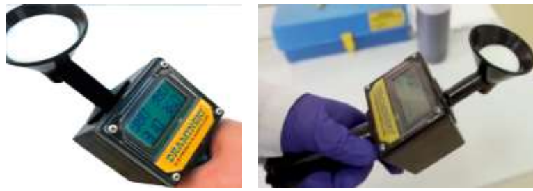
Figure 2. Draminski portable device for assessing milk conductivity
