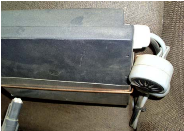
Figure 1. EDMeco recorder and electric flow meter
