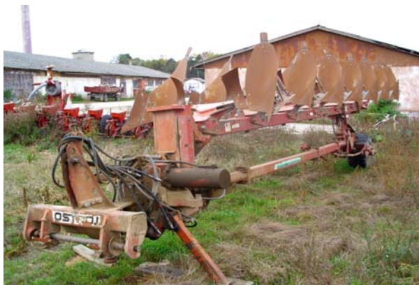
Figure 5. Rotating 7-mouldboard plow - Ostrój Opava
