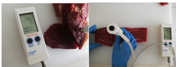
Figure 3. Laboratory pH meter, specially designed for the meat processing industry
