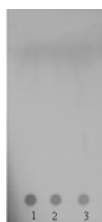
Figure 3. Pointing levan fractions eluted with Biogel P-200 column, 50-100 mesh, using a TLC Silica gel 60 plates
